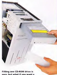
Fitting one CD-ROM drive is easy, but what if you want a CD-R in there too? Simple, just add another bay.
